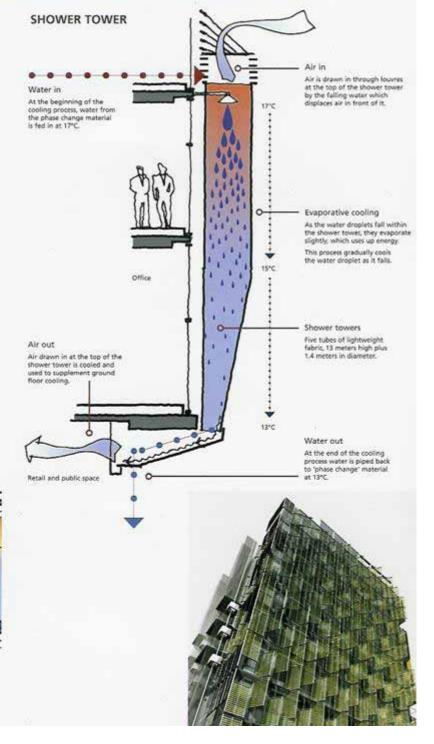
air falls within the towers it will be oled by evaporation from the water ower. The cool air will be channelled the shops below and the cool water pplied to a Phase Change Material CM) tank in the basement.
