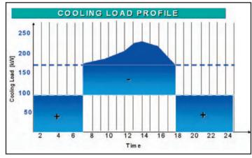
constant temperature. The biggest problem with water storage tanks is the stratification within the tanks during both charging and
