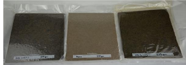
Once the PCM has been completely absorbed within the BoardICE sheets they can be cut and shaped to suit any applications. As the boards are loaded with non-water based organic solutions they tend to be waterproof. In principal, the boards can be manufactured as large as 1.22m (4') x 2.44m (8') dimensions and the standard thickness would be 12mm (1/2") and the relevant capacity, weight and cost details are attached in BoardICE table on the next page.
